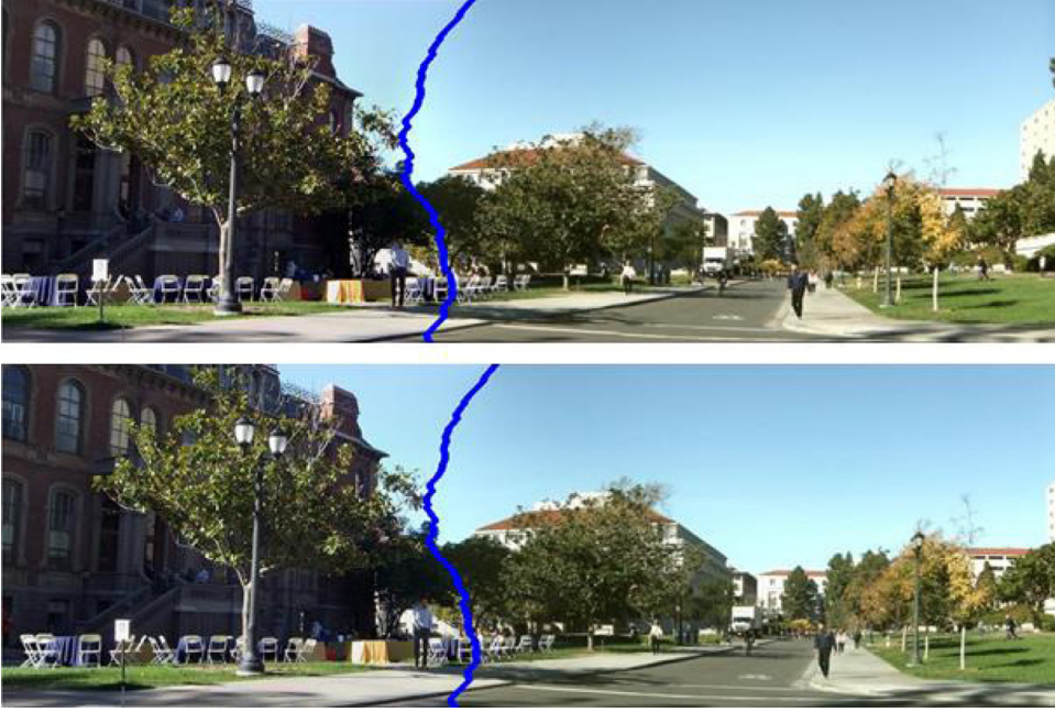
Fig. 5. Consistent seam. Top: seam in the stitched left view image; Bottom: seam in the stitched right view image.
